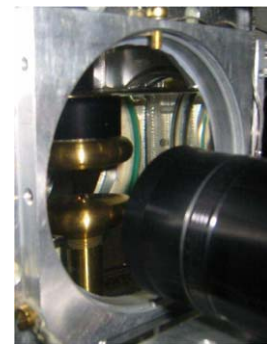
Fig. 5. Experimental set-up designed for visual observation of the behavior of water droplets in oil, exposed to the effect of an external electric field. (a) Sketch of the experimental set-up, (b) the set-up, (c) the test cell.
